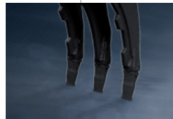
Optimized jaw shape for grasping stone
